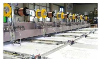
ZSK's Technical System CYCW 0600- placing and fixing conductive thread for automotive heating systems.
