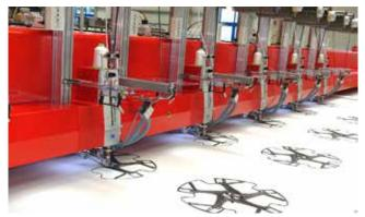
ZSK Technical System CZCW 0809- with eight W-Heads placing and fixing fibers.
