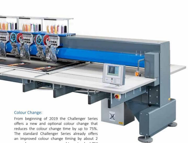
From beginning of 2019 the Challenger Series offers a new and optional colour change that reduces the colour change time by up to 75%. The standard Challenger Series already offers an improved colour change timing by about 2 seconds per process compared to a standard ZSK flat machine. The Challenger Series is equipped with a quicker catcher motor and the speed of the last stitches prior to a colour change, as well as the first stitches after a colour change have been improved.
