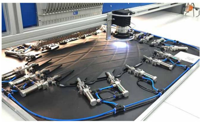
Machine: RACER 0124 with 24 needles and ZSK Vision System.
