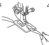
5. Lower the foot, then sew while lifting up the edge of the fabric to keep it feeding into the curl smoothly and evenly.
