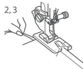
3. Sew 3 or 4 stitches while pulling the needle and bobbin threads.
